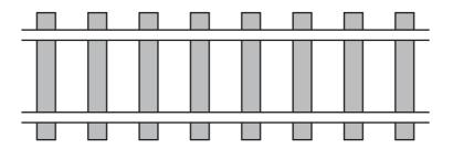
Originally, the sleepers were made from wood like oak, but in modern times they are made from concrete. As the wood rots, the oak sleepers are replaced with concrete ones. Each 10 km section is replaced over a period of 3 months. There are 2400 sleepers per km of track.
